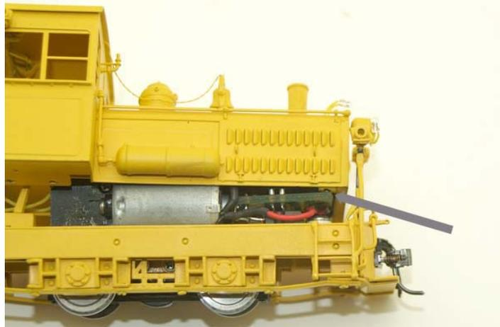
Figure 7. When removing the shell be careful not to hit the radiator and the circuit board
