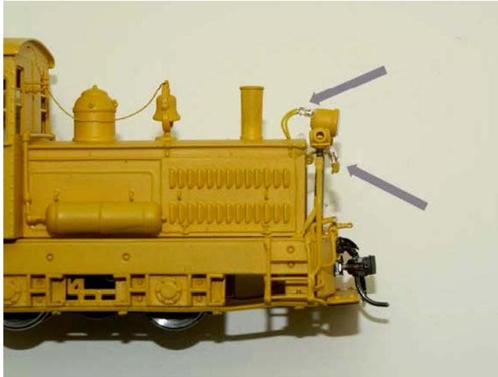
Figure 5. Removing the bulbs from the head light and front marker lights
