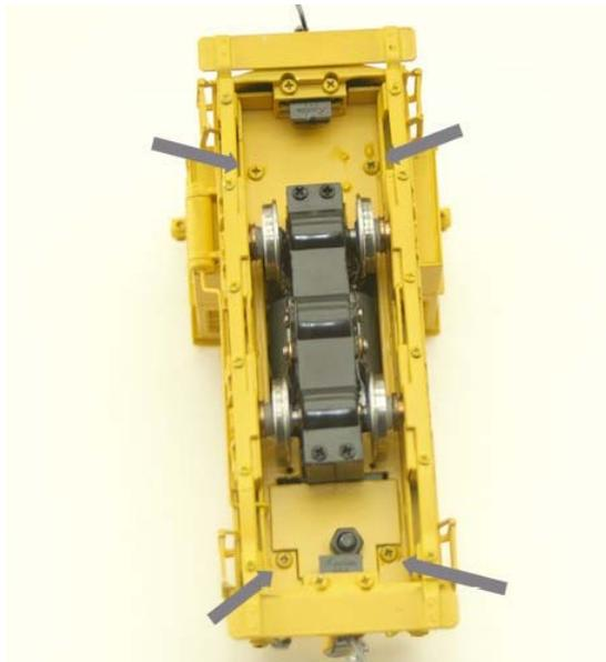
Figure 6. The screws that hold the shell to the frame
