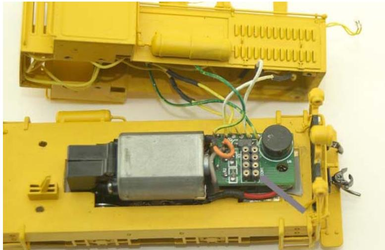
Figure 8. Decoder alignment.
