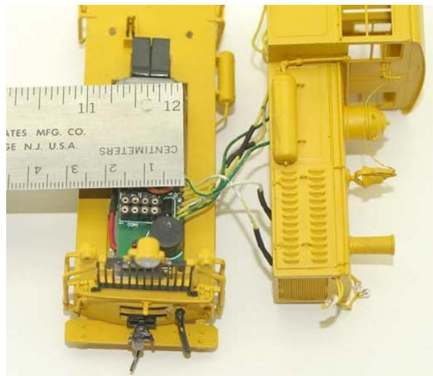
Figure 3. The overall width and socket position of an integrated socket decoder
