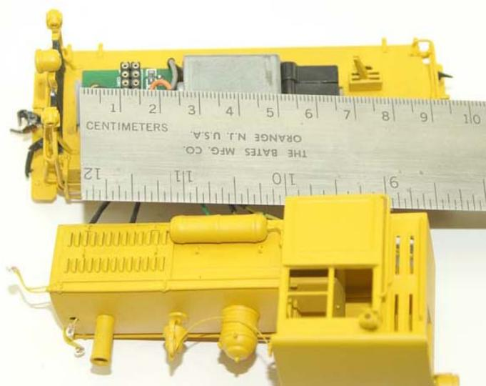
Figure 2. The overall length and socket position of an integrated socket decoder
