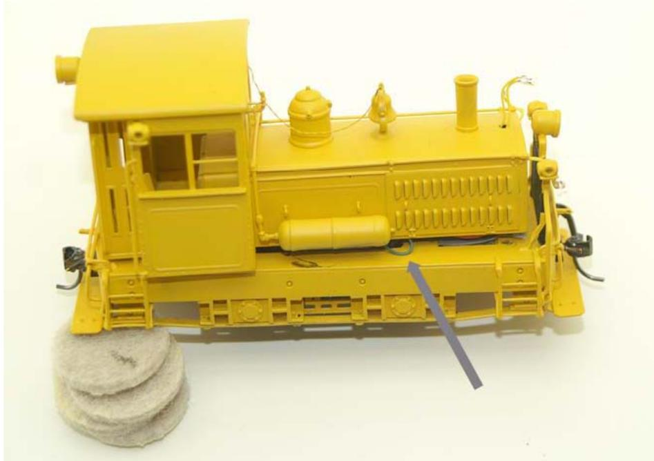
Figure 9. When replacing the shell watch for stray wires
