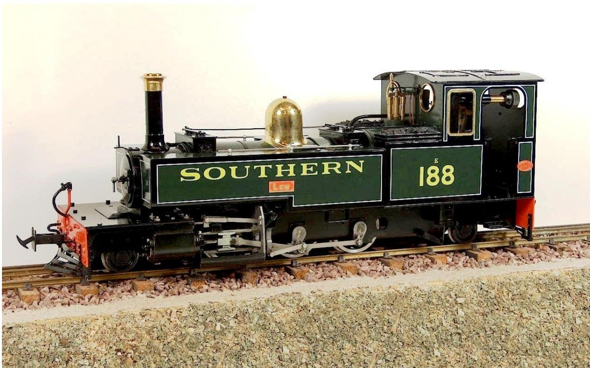
Lew was built in 1925 to a similar design to the previous Manning Wardle locomotives constructed for the Lynton & Barnstaple Railway, the main difference being a redesigned cab to eliminate a smoke trap, and give more room to the crew.
