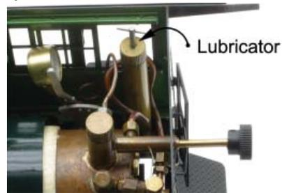
4. Unscrew the filler plug and fill the boiler to the top with water then pull out 40 ml with large syringe. Use only distilled water in your engine's boiler. Tap water contains minerals that will leach out and ultimately affect the performance of the engine.
