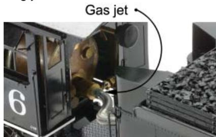
3. The displacement lubricator is in the cab. This lubricator ensures the cylinders and valves are properly lubricated inside. As the steam passes through it, a small amount will condense into wa-
