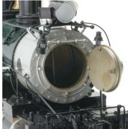
The fire should flash back into the back of the flue with a quiet "pop". If it wants to burn in the smokebox or in the forward part of the flue, slowly close the gas valve until it flashes back to the burner. Don't let the fire burn in the smokebox - your engine
