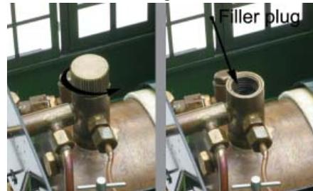
5. Finally, add fuel. Your C-19 burns butane gas. The gas tank is located in the tender beneath the dummy coal load. Remove the coal load with the ring provided. Butane gas can be
