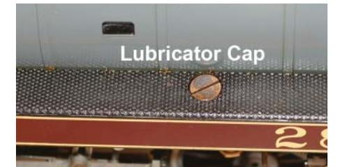
Remove the lubricator cap and draw out any water from the previous run with a syringe. Use only proper steam cylinder oil. Fill the lubricator, but leave a small air space between the oil and the cap.
