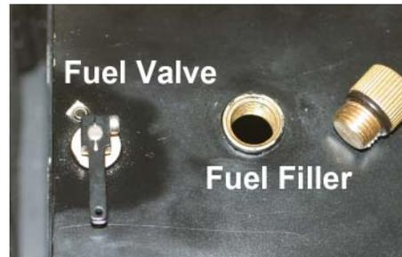
When fueling the locomotive the fuel valve should be shut. Replace filler cap immediately after filling tank. The alcohol will cause the O-ring to dry out, use a small drop of machine oil on the O-ring to keep it pliable.
